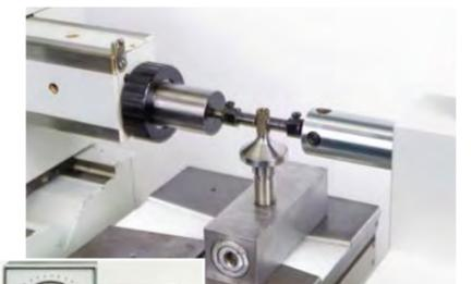
横型測長機 Length measuring machine
